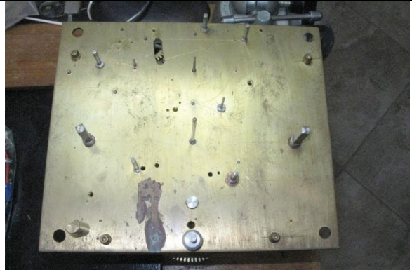
WNS-CLK-182 – Front Plate with Layout Scribe Markings
