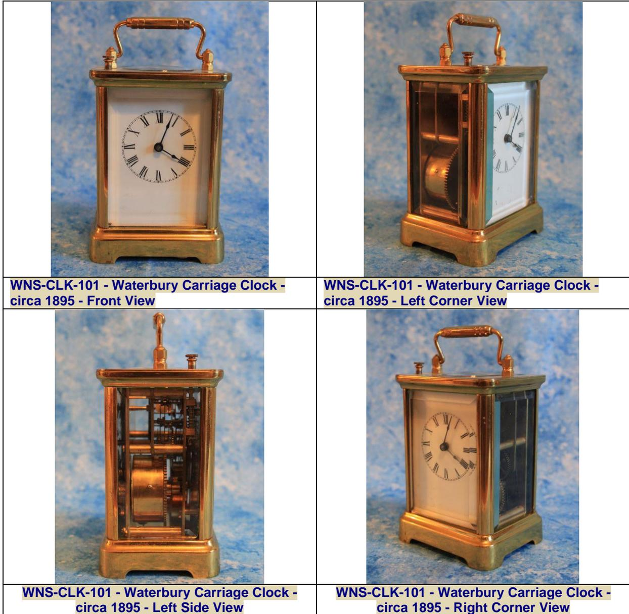
**Waterbury Clock Company - Brass and Glass Carriage Clock - Mechanical 8-day movement with strike and chime winders - hour repeating function and hour and 1/2 hour gong. Marked on the movement plate 'Pat'd JAN 13 91 [1891]' and 'Waterbury Clock Co. U.S.A.' and marked on the back door 'PATENTED DEC. 23, 1890 and JAN. 13, 1891'. 4-3/8" tall x 2-1/4" wide x 2-3/4" long (Circa 1895).**
