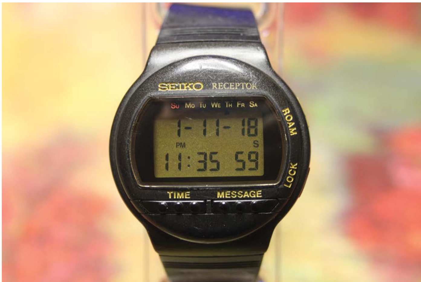
Figure 3. Seiko Receptor includes paging and messaging services and an embedded antenna in the wrist band, circa 1990. AUTHOR'S COLLECTION.
