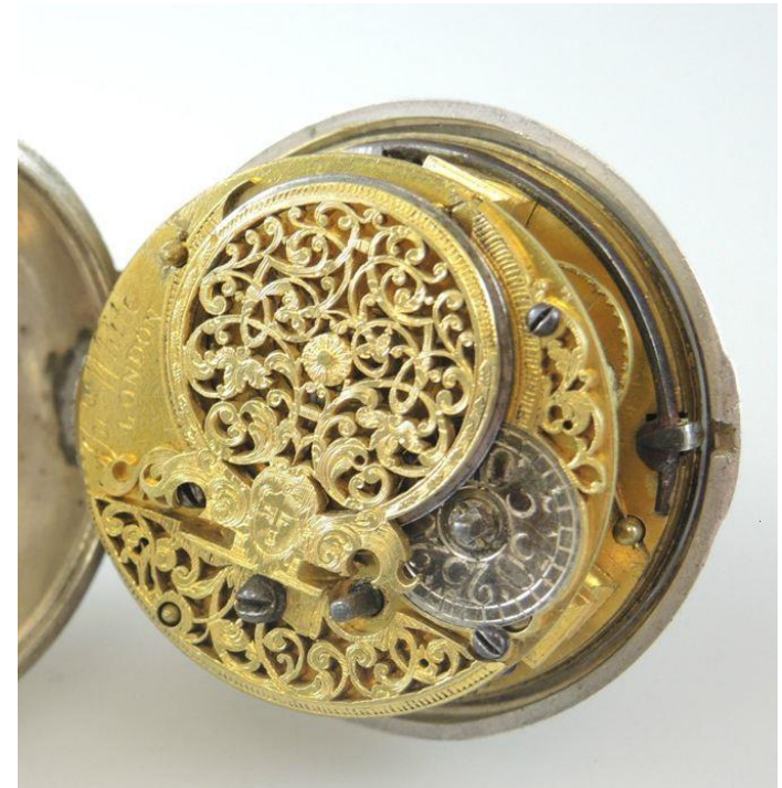
Right: Circa 1690 - Maker: John White - Movement – the large gilt full plate verge movement has large Egyptian style pillars and an oversized watch cock, which is decorated with fine piercing and features finely engraved cherubs.
