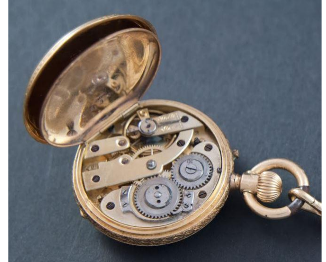
Right: Cylinder escapement - movement - Joseph French - London (circa 1850).
