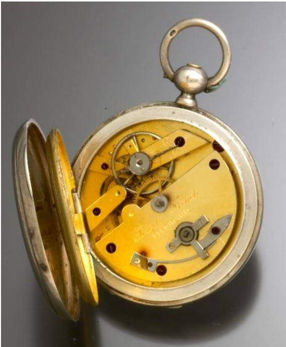
Right: Cylinder escapement - movement - Joseph French - London (circa 1850).
