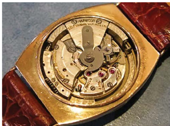
Figure 3. The Harwood self-winding (automatic) wristwatch, ca. late 1920s, movement view. Made in Britain. Accessed May 13, 2016. http://madeupinbritain.uk/Automatic_watch
