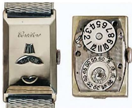
Figure 5. The Cortebert jump-hour wristwatch. The front case and rotating disks on the movement views, ca. 1920s. Unique Watch Guide. Accessed June 6, 2016. http://www.uniquewatchguide.com/mechanical-digital-watches.html
