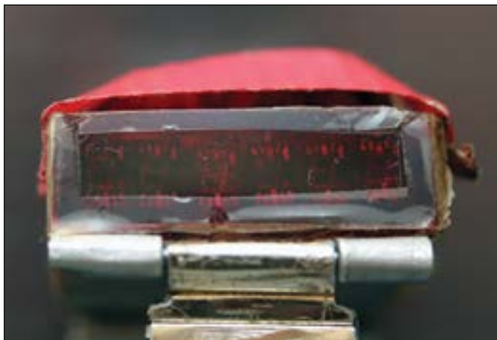
Figure 7. Roger W. Riehl's solar-powered wristwatch prototype with digital display view, ca. 1968-1970.
