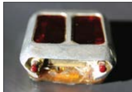
Figure 9. Roger W. Riehl's solar-powered wristwatch prototype with the two push-button control design that failed waterproof testing, ca. 1970.
