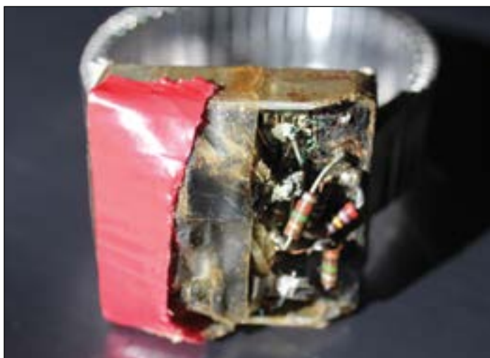
Figure 8. Roger W. Riehl's solar-powered wristwatch prototype's top view with circuitry exposed, ca. 1968-1970.
