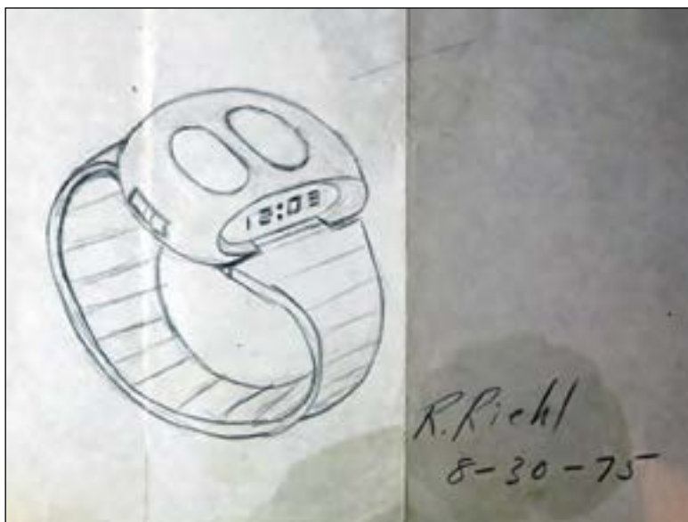
Figure 13. Roger W. Riehl's hand drawing of a Synchronar concept wristwatch with a cushion-style case and oval solar panels, ca. 1975.
