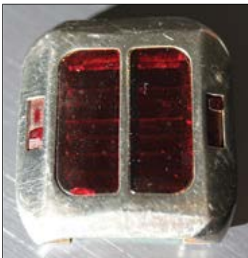
Figure 11. Roger W. Riehl's solar-powered wristwatch prototype with waterproof slider controls on the top of the case, ca. 1971-1972.
