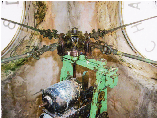
Figure 3. Original Seth Thomas movement with the electric motor running in the clock room. PHOTO COURTESY OF TOM BRANSFORD AND CHAPTER 154.
