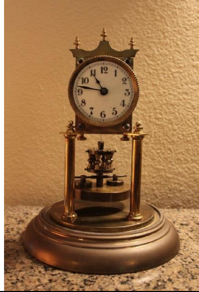
WNS-CLK-135 - Jahresuhren - Disk Pendulum 400 day clock - circa 1912 - Full Front View without the glass dome
